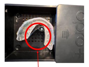
Use adjustable arms to secure the mouthguard against the charging coil. Position of arms can be adjusted if needed by loosening screw. Arms should push the mouthguard as close to the coil as possible.
