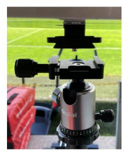
Position the receiver on its tripod around from the centre line of the pitch with the direction label facing the field of play about 1-2m back from the side line or athlete participation area.
