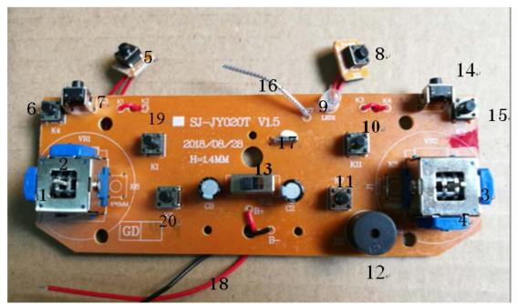
1 and 2: Throttle potential controller and left and right steering potential controller
