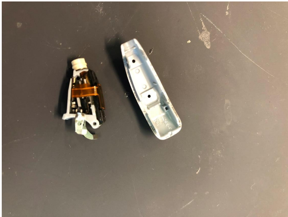
Earpiece PCB Removed from Folding Frame
