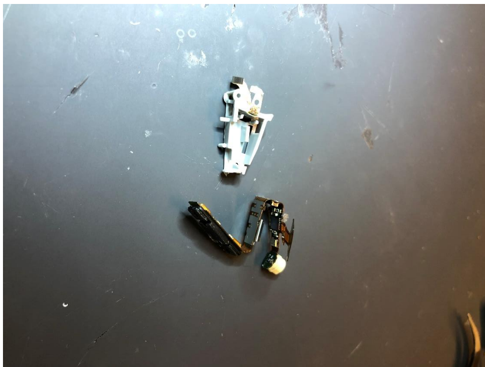
Earpiece PCB Removed from Folding Frame
