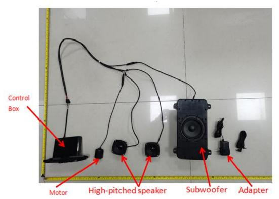
The system consists of left and right channels of high quality speakers, a main control box, a charger, a motor, Audio line.
