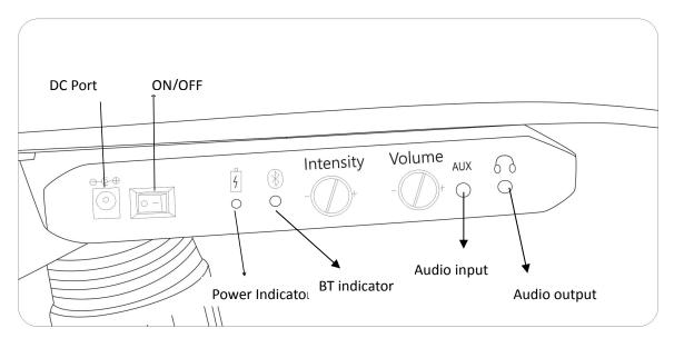
STEP 1: Plug the adapter output into the 'DC PORT'and plug the adapter into the home outlet.
