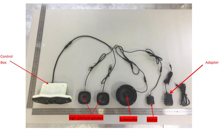
The system consists of left and right channels of high quality speakers, a main control box, a charger, a motor, Audio line.
