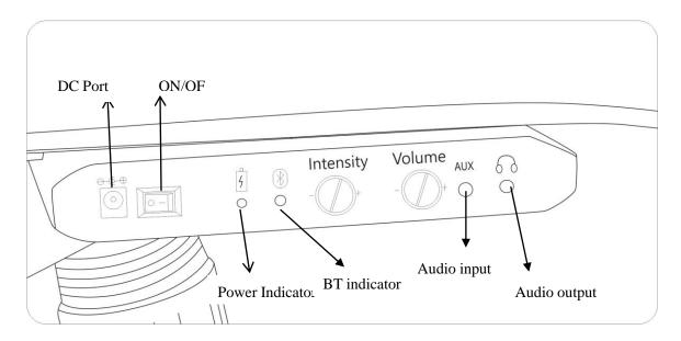
STEP 1: Plug the adapter output into the 'DC PORT'and plug the adapter into the home outlet.
