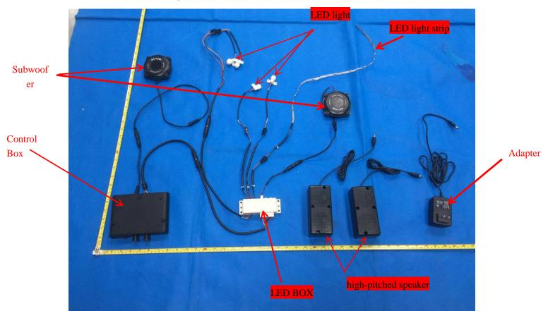
The system consists of left and right channels of high quality speakers, a Bluetooth power amplifier board, a charger, LED Control box, LED light strip.
