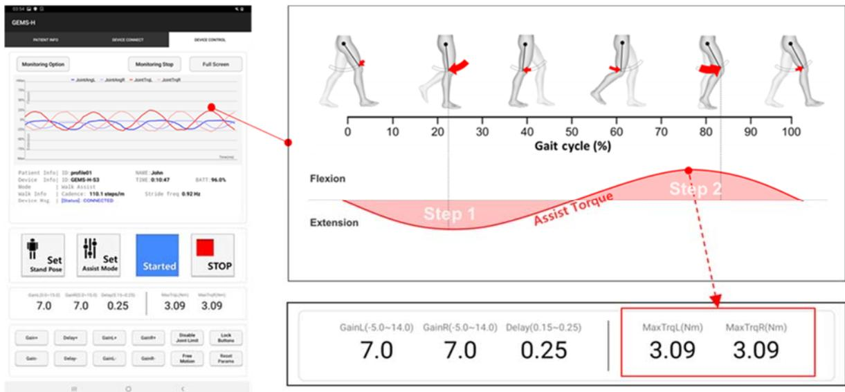
Users can monitor the maximum assistive torques that the device delivers to the patient as the user changes the assist gain. The maximum assistive torques MaxTrqL and MaxTrqR indicate the maximum values of assistive torques provided by the device for the last two steps. Even with parameters fixed, the assistive strength will vary based on the patient walking condition such as step length, walking speed, and other factors.
