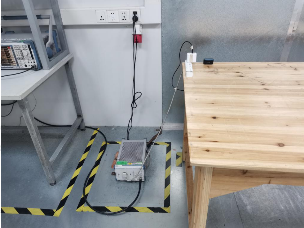
Photo of Conducted Emission Measurement
