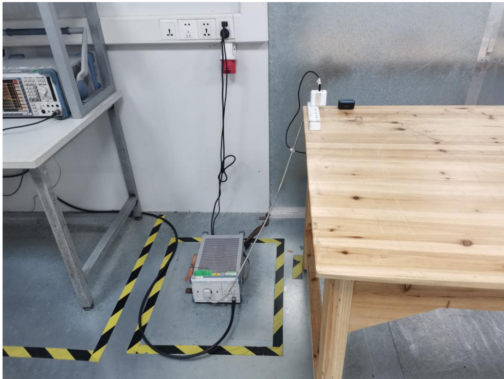
Photo of Conducted Emission Measurement
