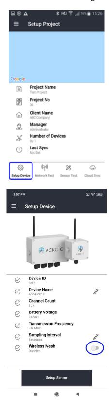
(iii) <Optional Step> If Wireless Mesh (Relay) function is to be deployed, click on "Wireless Mesh" toggle button to enable. Once done, click on "Setup Sensor", you can now configure the sensor settings.
