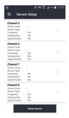
(v) **Sensor Code**: Your desired sensor name. **Sensor Type**: Select respective sensor type. **Parameters**: Turn on the parameters as connected to the Node. **Mode**: Please select the respective Sweep Mode (A or B or C), depending on the sensor.
