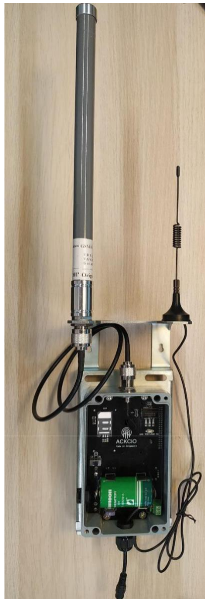
Gateway antenna & Cellular (GSM) antenna positioning - left and right respectively
