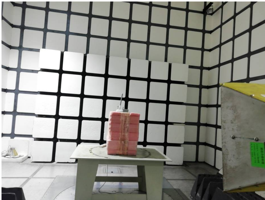
Radiated Emissions View (Above 1 GHz)
