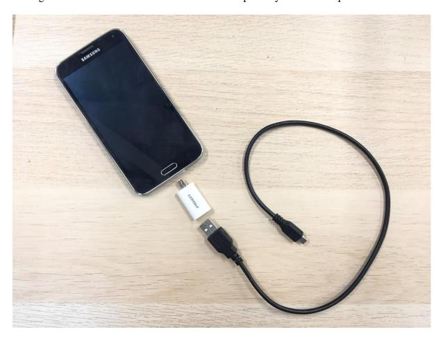
3. Important! Please make sure the Node is switch off before connecting to your Android phone. 4. Plugin micro USB end to the Node.
