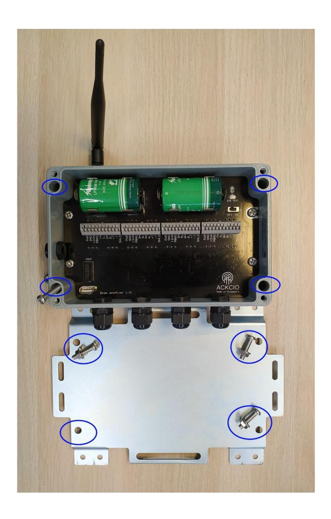
Use four screws and nuts to attach the node to the bracket
