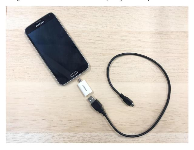
3. *Important!* Please make sure the Node switch is turned off before connecting to your phone. 4. Plugin micro USB end to the Node.
