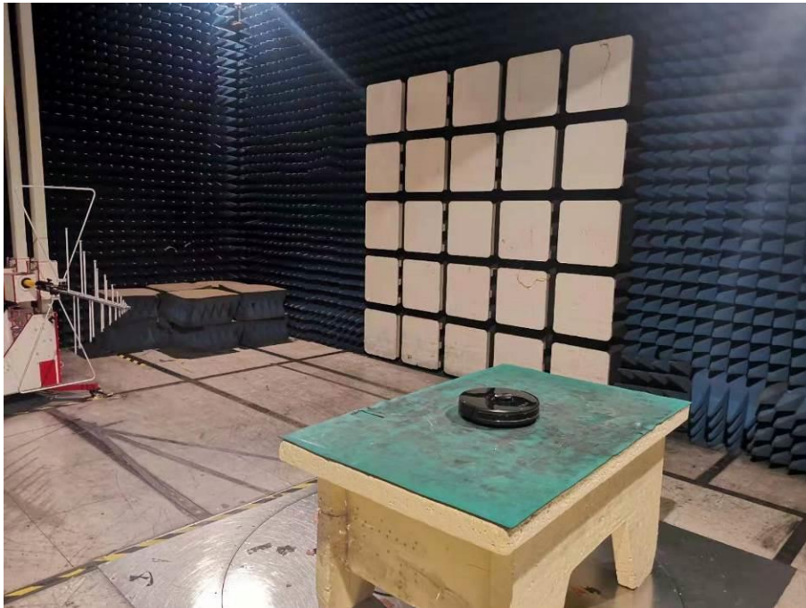
Spurious Emission Test Setup (Below 1GHz)
