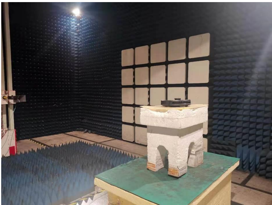
Spurious Emission Test Setup (Above 1GHz)
