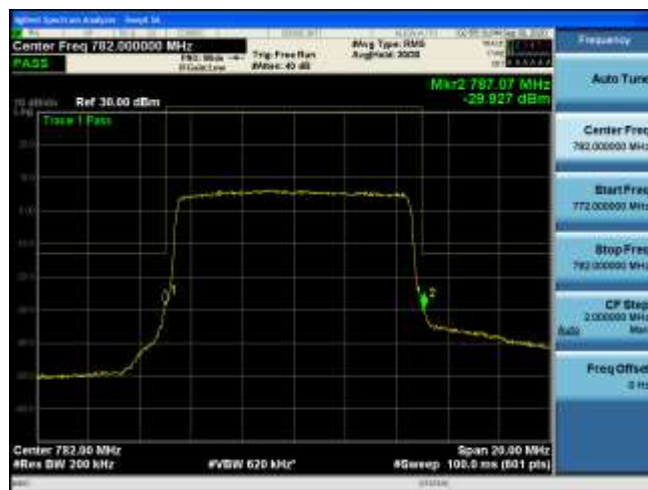
High Band edge RB Size 50, RB offset 0
