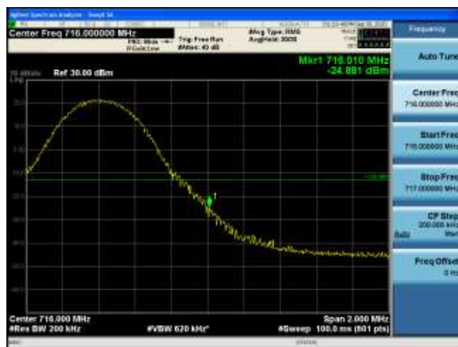
High Band edge RB Size 50, RB offset 0
