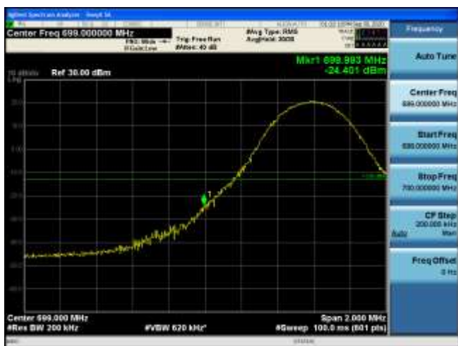
Low Band edge RB Size 50, RB offset 0
