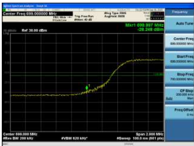
Low Band edge RB Size 50, RB offset 0
