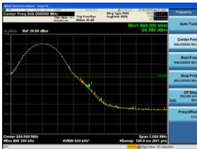
High Band edge RB Size 50, RB offset 0
