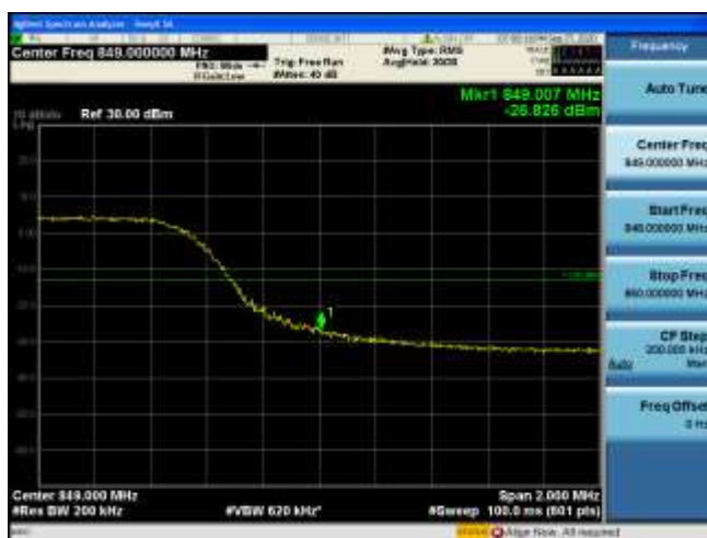
High Band edge RB Size 50, RB offset 0
