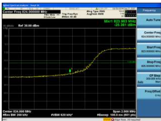
Low Band edge RB Size 50, RB offset 0
