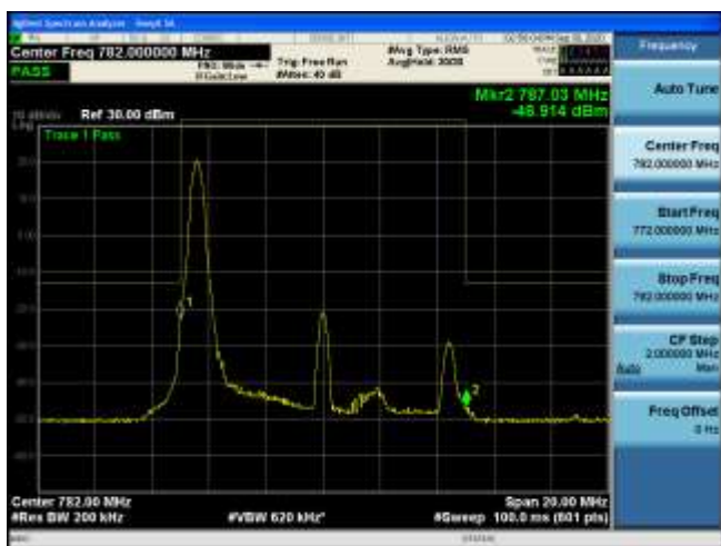
Low Band edge RB Size 50, RB offset 0
