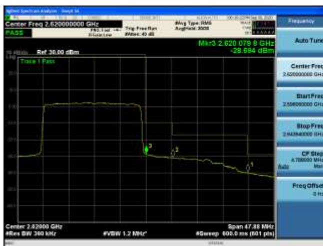
High Band edge RB Size 100,RB offset 0
