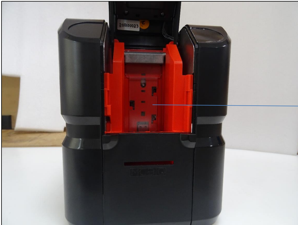
MC310 printer front view showing Card tray
