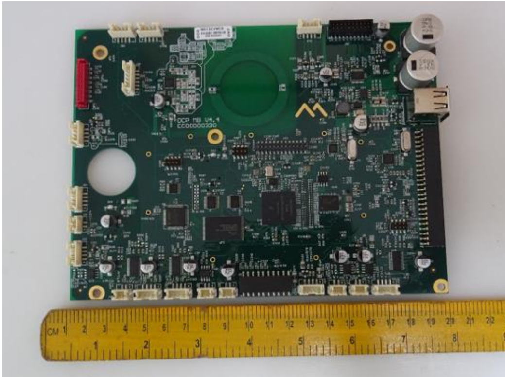
Printer main board Dimensional view (Width)
