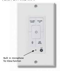
Turn the power on by pressing the center button. Center LED lit button will light in default as green which indicates it is in the WIFI mode. If the unit has the "Mode" button pressed it will toggle the mode to Bluetooth mode, which will change the center button to blue color. With the device in the WIFI mode open you will hear two audible beeps. Make sure you wait for the second audio beep. Now open the MUZO player on your device.
