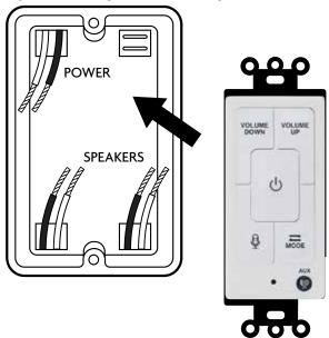
Wires from 24 volt, 3 amp power source, and speaker wires led through standard "J" box.
