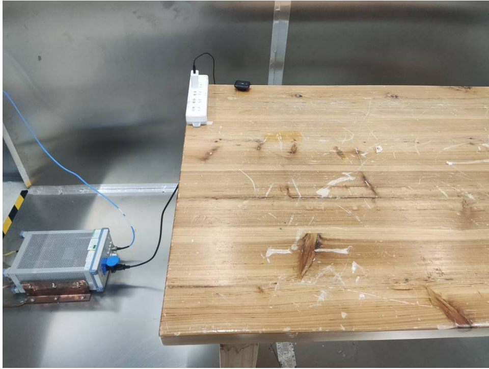
Photograph 3: Set-up for Conducted Emission on AC Mains
