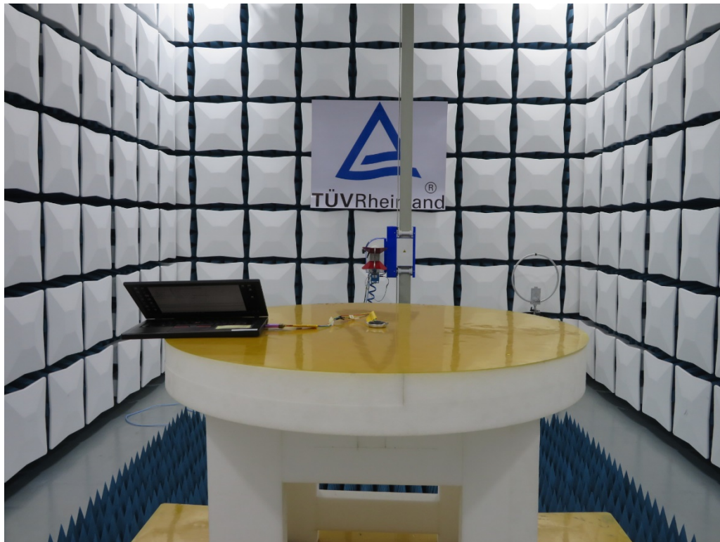
Photograph 2: Set-up for Radiated Spurious Emission, Above 1GHz
