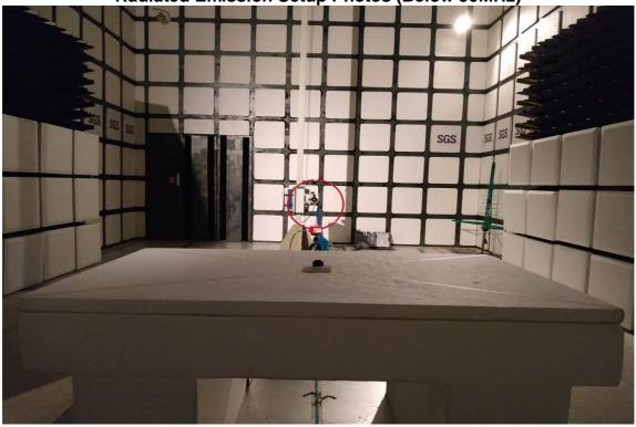
Radiated Emission Setup Photos (30MHz~1GHz)
