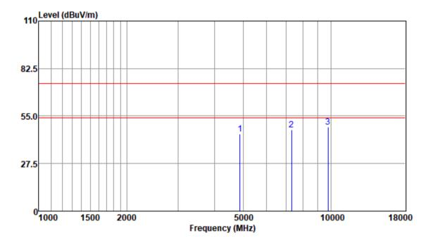
Test Mode: 01; Polarity: Horizontal; Modulation:GFSK; Channel:middle
