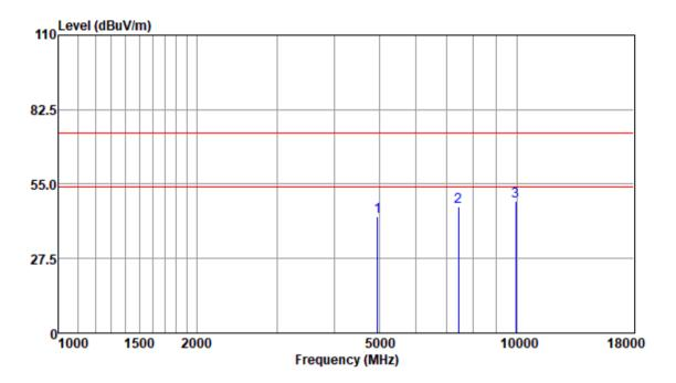
Test Mode: 00; Polarity: Horizontal; Modulation:GFSK; Channel:High
