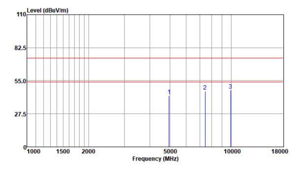
Test Mode: 01; Polarity: Vertical; Modulation:GFSK; Channel:High
