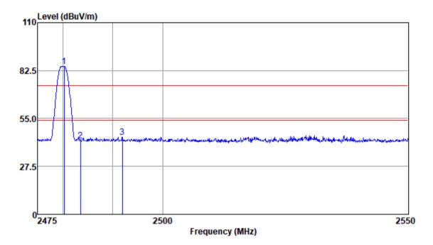
Test Mode: 00; Polarity: Vertical; Modulation:GFSK; Channel:High
