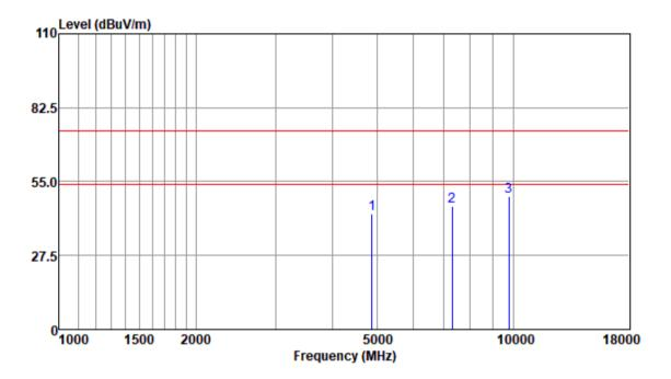
Test Mode: 01; Polarity: Vertical; Modulation:GFSK; Channel:middle
