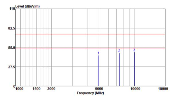
Test Mode: 00; Polarity: Vertical; Modulation:GFSK; Channel:High
