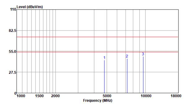
Test Mode: 01; Polarity: Horizontal; Modulation:GFSK; Channel:Low
