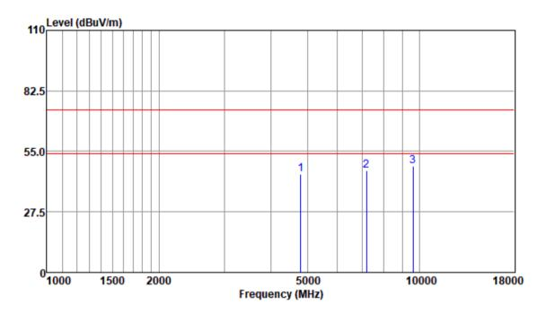
Test Mode: 00; Polarity: Vertical; Modulation:GFSK; Channel:Low
