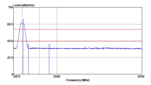
Test Mode: 01; Polarity: Vertical; Modulation:GFSK; Channel:High
