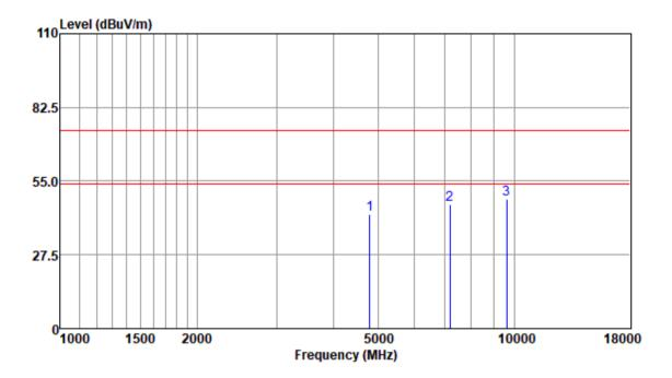
Test Mode: 01; Polarity: Vertical; Modulation:GFSK; Channel:Low
