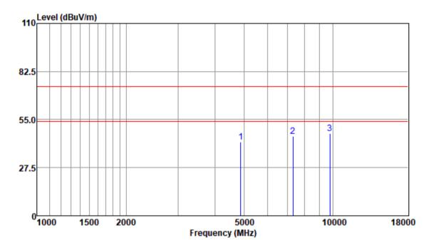
Test Mode: 00; Polarity: Vertical; Modulation:GFSK; Channel:middle
