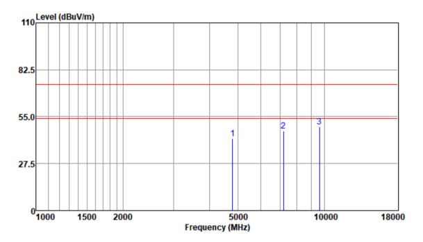
Test Mode: 00; Polarity: Horizontal; Modulation:GFSK; Channel:Low
