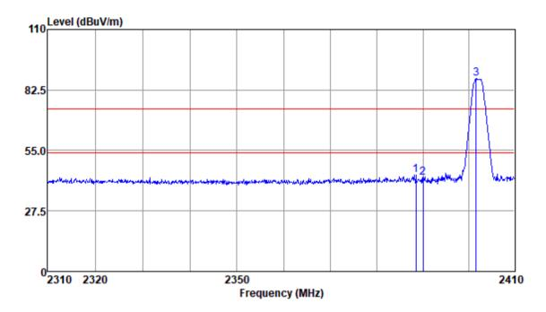
Test Mode: 01; Polarity: Vertical; Modulation:GFSK; Channel:Low
