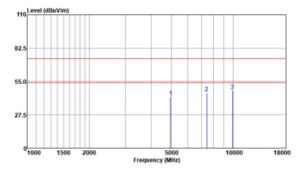
Test Mode: 01; Polarity: Horizontal; Modulation:GFSK; Channel:High
