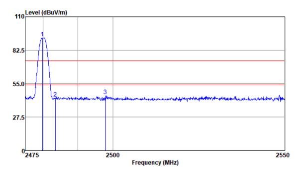
Test Mode: 00; Polarity: Horizontal; Modulation:GFSK; Channel:High
