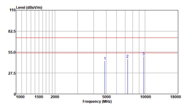
Test Mode: 00; Polarity: Horizontal; Modulation:GFSK; Channel:middle
