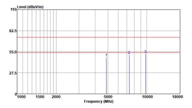
Test Mode: 01; Polarity: Horizontal; Modulation:GFSK; Channel:middle
