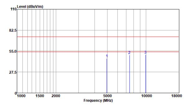
Test Mode: 01; Polarity: Horizontal; Modulation:GFSK; Channel:High
