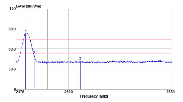
Test Mode: 01; Polarity: Vertical; Modulation:GFSK; Channel:High
