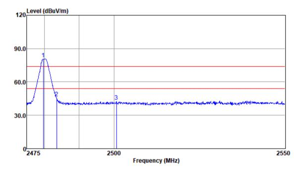
Test Mode: 00; Polarity: Vertical; Modulation:GFSK; Channel:High
