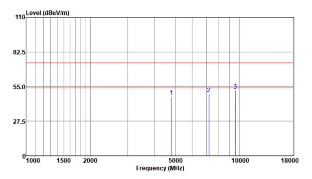
Test Mode: 00; Polarity: Vertical; Modulation:GFSK; Channel:Low
