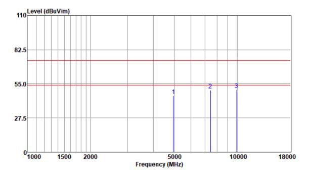
Test Mode: 00; Polarity: Horizontal; Modulation:GFSK; Channel:High
