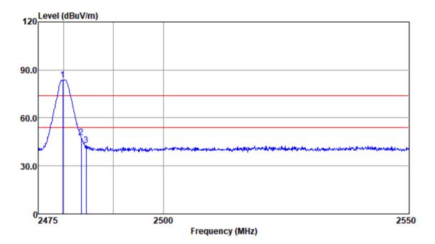
Test Mode: 00; Polarity: Horizontal; Modulation:GFSK; Channel:High
