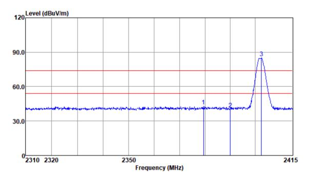
Test Mode: 01; Polarity: Horizontal; Modulation:GFSK; Channel:Low
