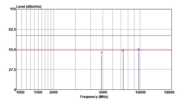
Test Mode: 01; Polarity: Vertical; Modulation:GFSK; Channel:middle
