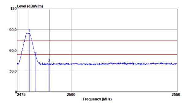
Test Mode: 01; Polarity: Horizontal; Modulation:GFSK; Channel:High
