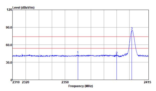
Test Mode: 00; Polarity: Vertical; Modulation:GFSK; Channel:Low
