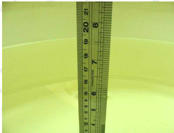
Photo of Liquid Height for Body SAR
