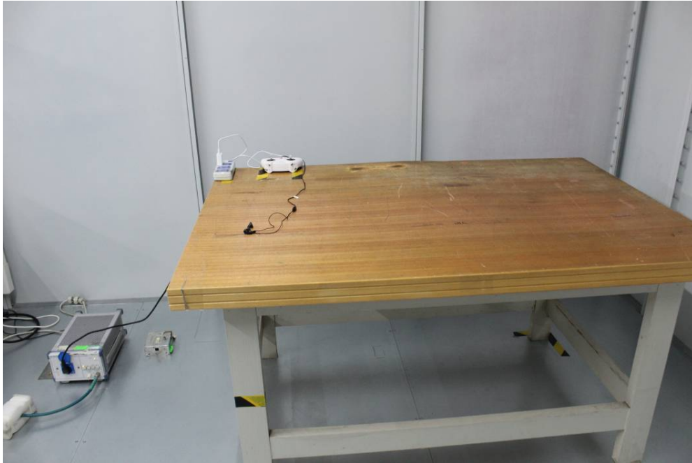
Conducted Emissions - Front View
