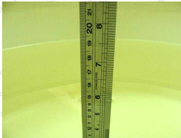
Photo of Liquid Height for Body SAR
