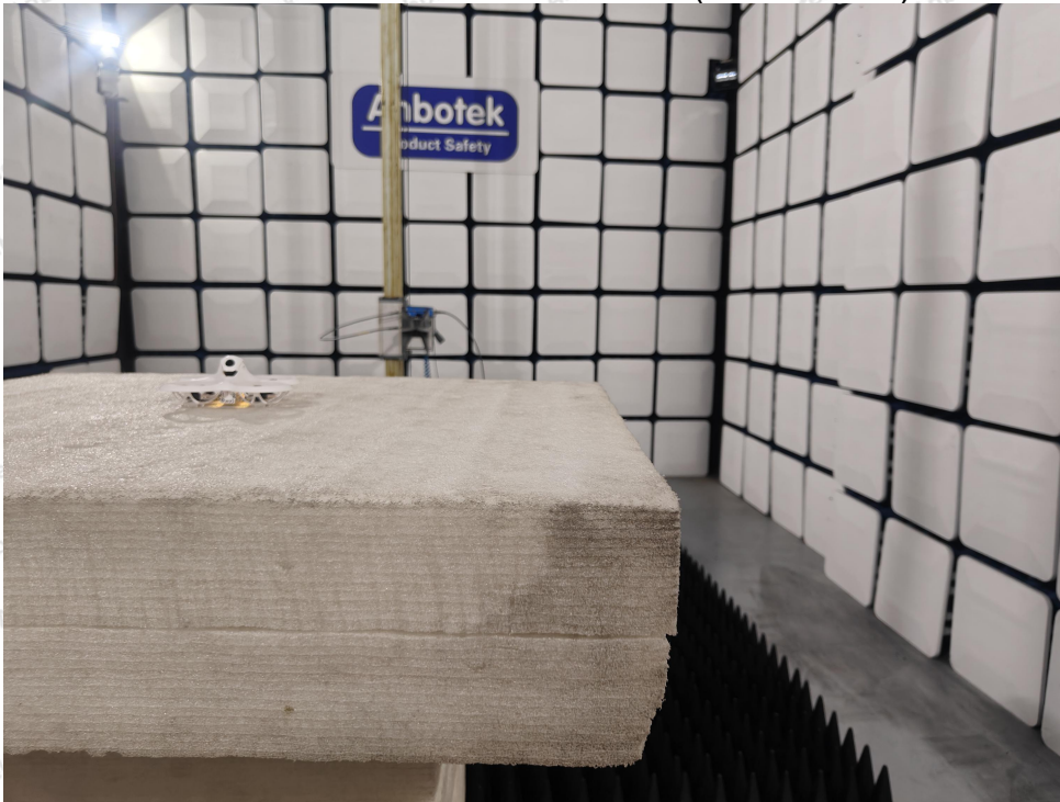
Photo of Radiation Emission Test (above 1GHz)
