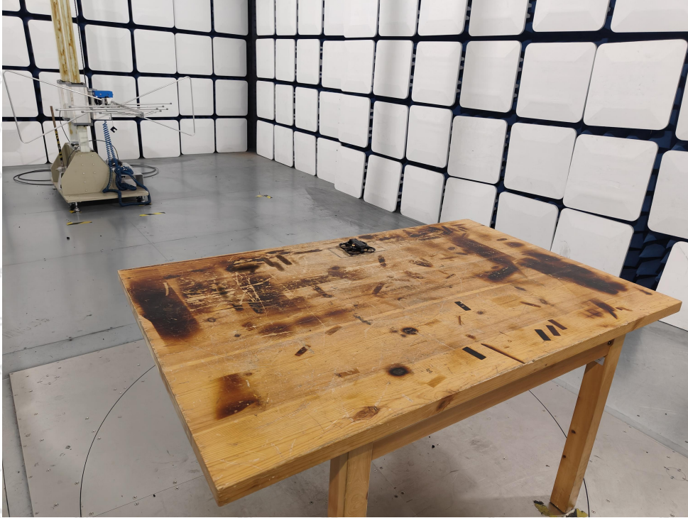
Photo of Radiation Emission Test (below 1GHz)
