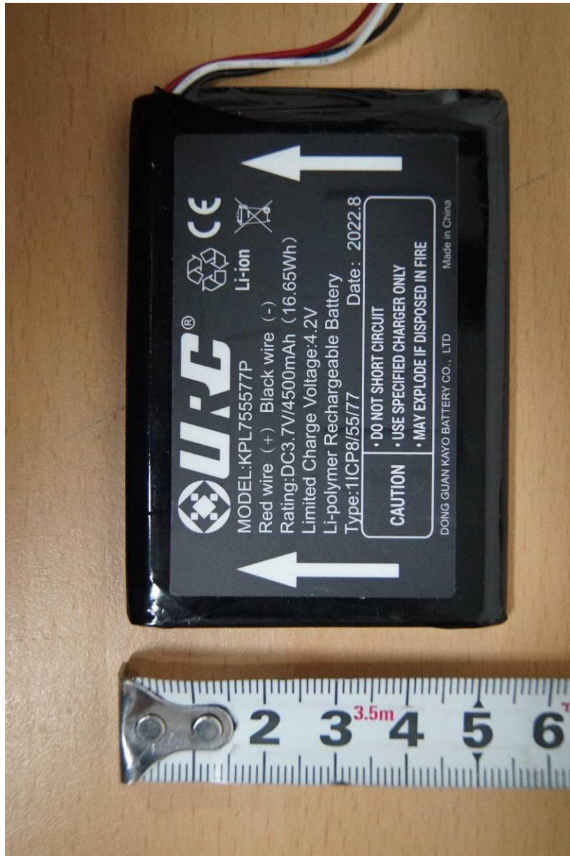
< Battery Top view >
