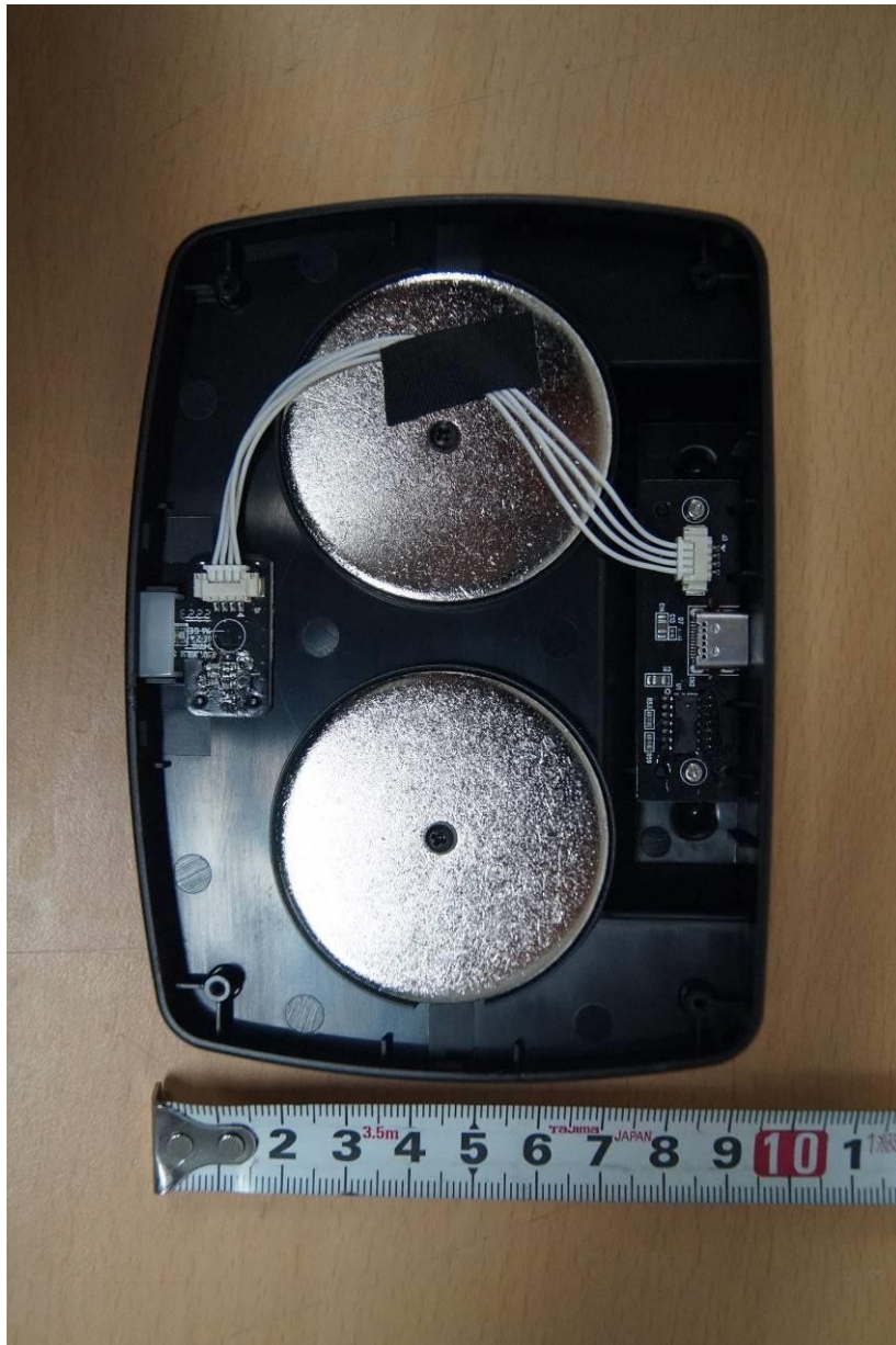
< Charging cradle inside view >
