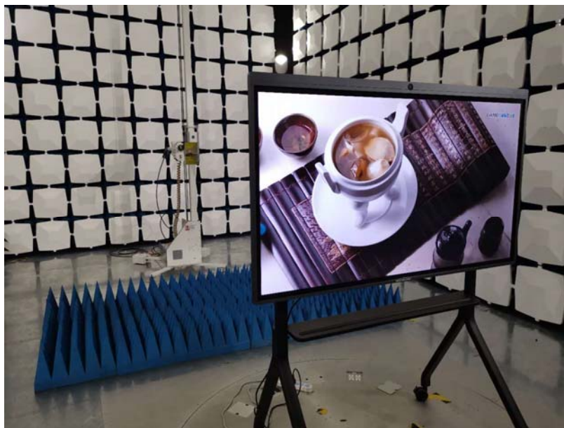
Above 1GHz for radiated emission test setup
