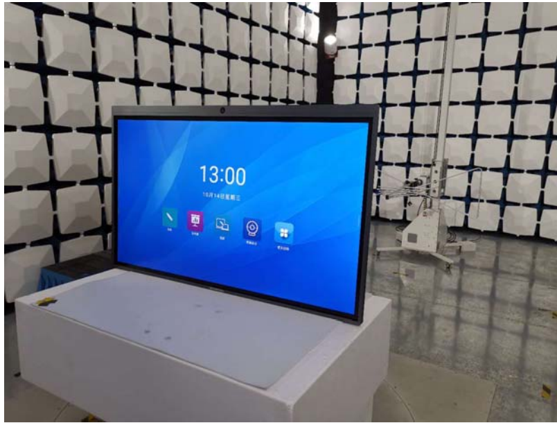
Blow 1GHz for radiated emission test setup
