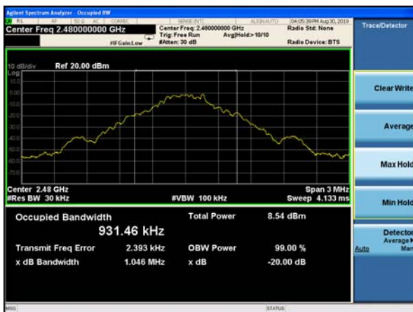
20dB Bandwidth plot on channel 78 (1Mbps)
