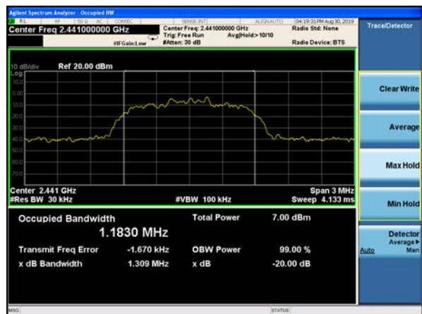
20dB Bandwidth plot on channel 78 (2Mbps)
