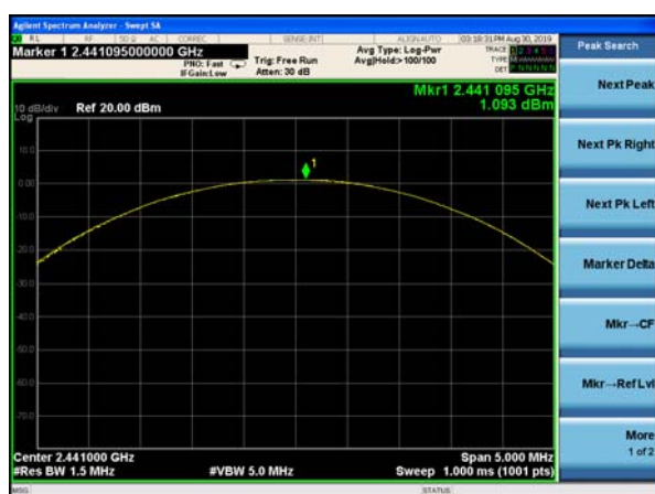
Peak output Power plot on channel 39 (3Mbps)
