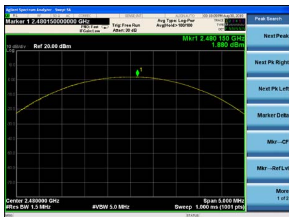
Peak output Power plot on channel 78 (3Mbps)
