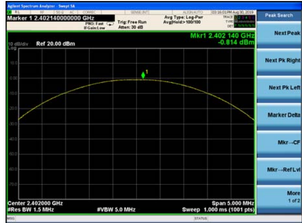
Peak output Power plot on channel 39 (2Mbps)
