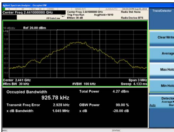
20dB Bandwidth plot on channel 78 (1Mbps)
