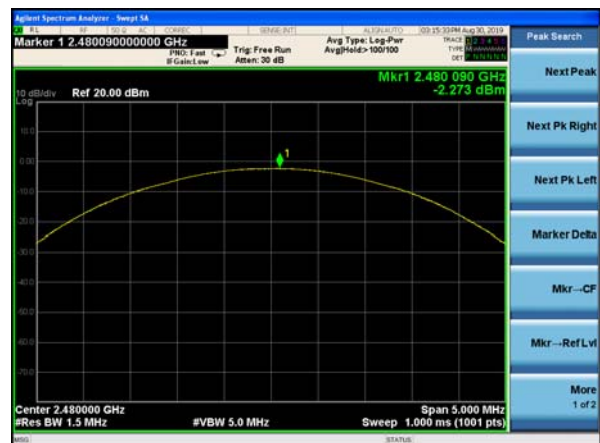
Peak output Power plot on channel 78 (2Mbps)
