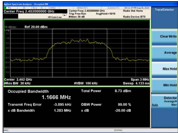
20dB Bandwidth plot on channel 39 (2Mbps)
