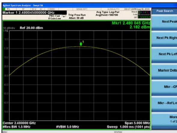
Peak output Power plot on channel 78 (1Mbps)
