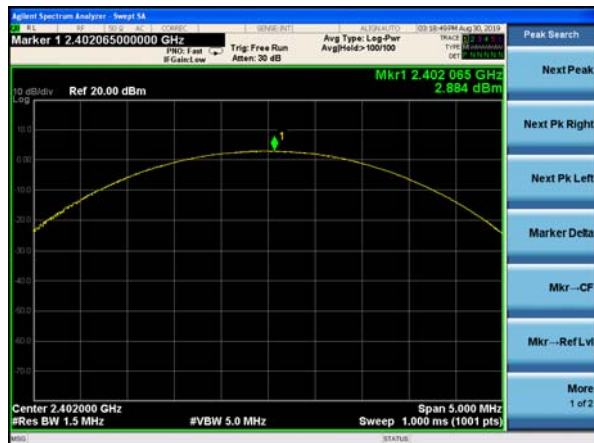
Peak output Power plot on channel 39 (3Mbps)
