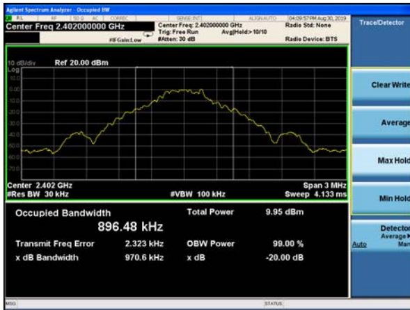
20dB Bandwidth plot on channel 39 (1Mbps)
