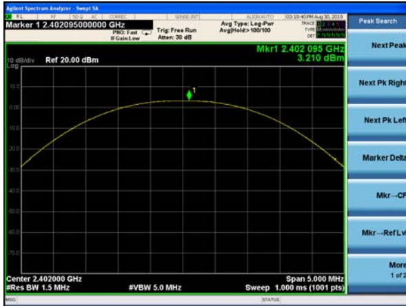
Peak output Power plot on channel 39 (1Mbps)
