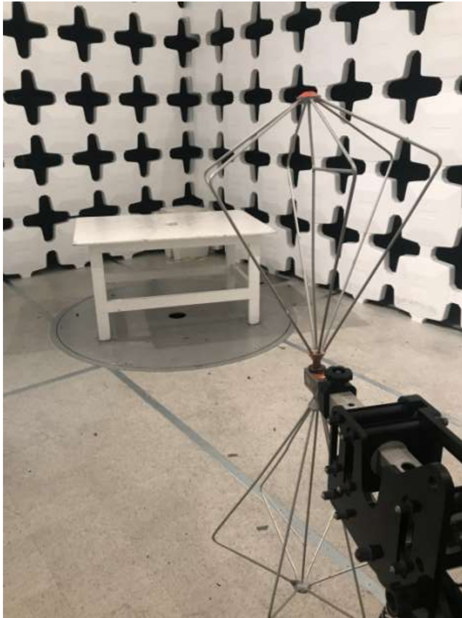
Figure 3. Radiated Emissions, 30 MHz - 200 MHz
