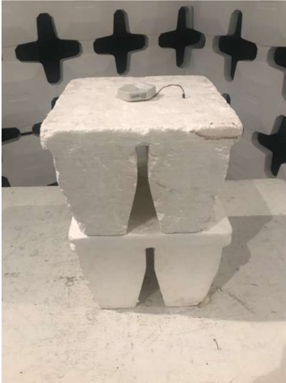
Figure 6. Radiated Emissions Test Setup above 1 GHz (intentional emissions)
