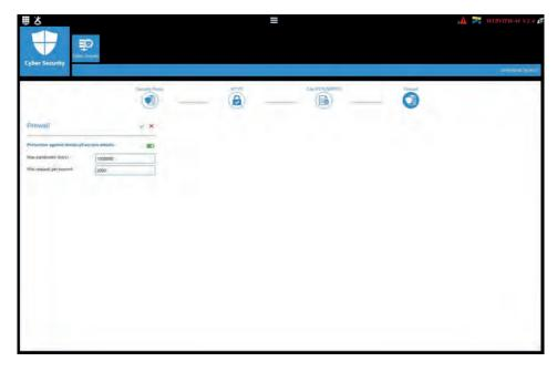
A client exceeding one of the above parameters while communicating to the DIRIS Digiware M-50/M-70 gateway will be blocked for 30 seconds.
