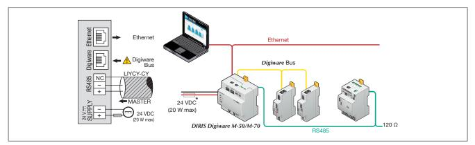
(\*) If the 24 VDC power supply is not provided by Socomec, a 1 A / 24 VDC fuse must be used. For North America, the use of recognized fuses is mandatory.
