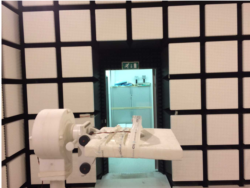
Photo 5 - RSE Setup > 1000 MHz
