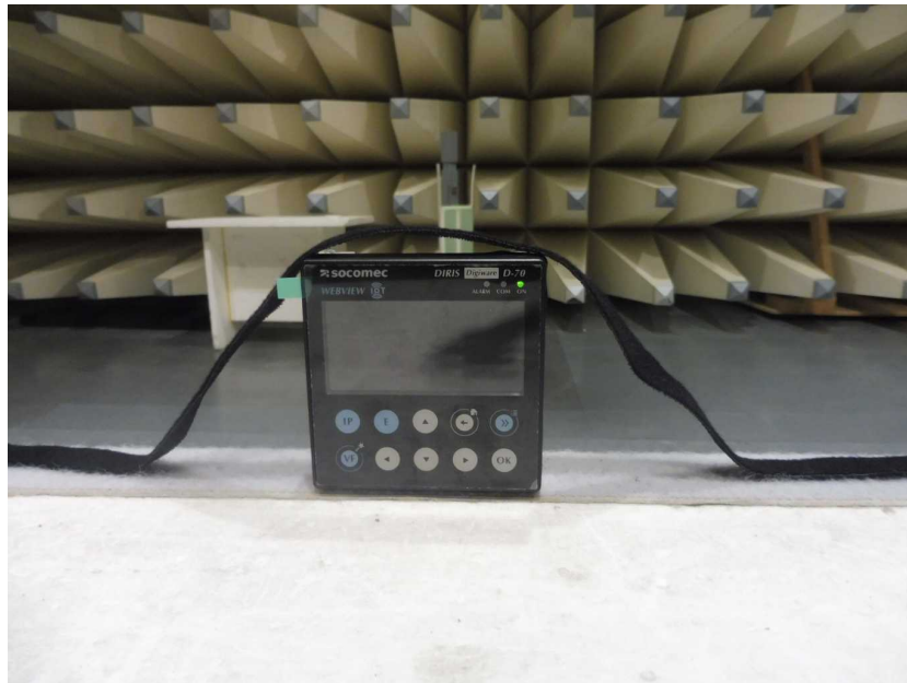
Photo 1 - RSE Setup 30 MHz to 1000 MHz
