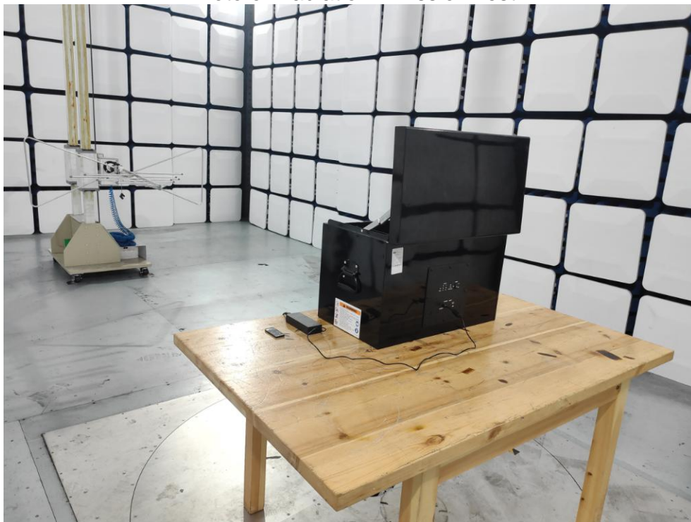
Photo of Radiation Emission Test
