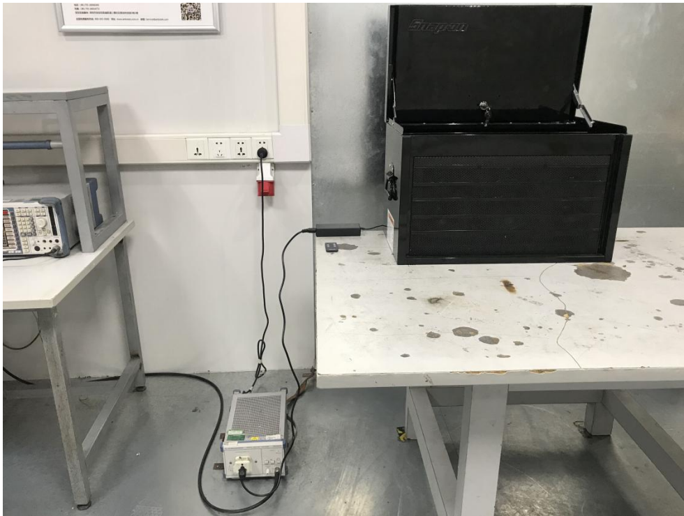
FCC ID: 2AT5Z-KRA4059 Photo of Conducted Emission Measurement
