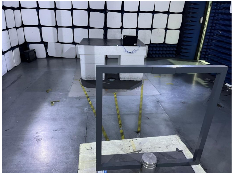
Radiation Emission Test Setup (Below 30MHz)
