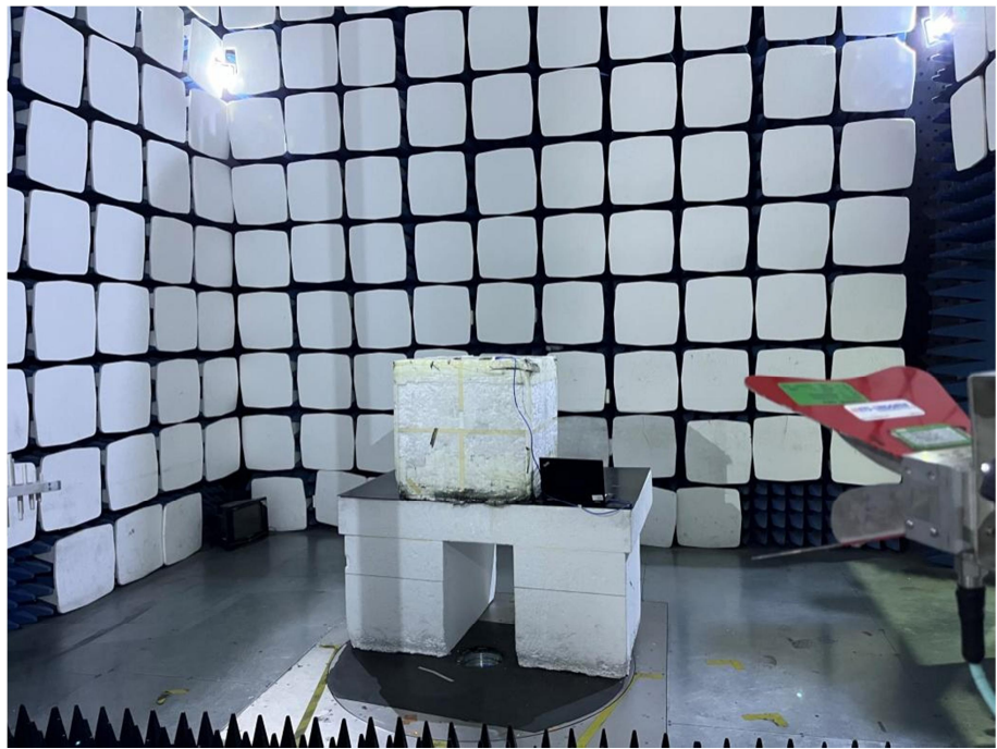
Radiation Emission Test Setup (1GHz to 18GHz)
