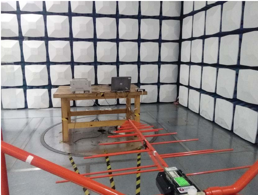
Radiated Emission Below 1GHz Rear View
