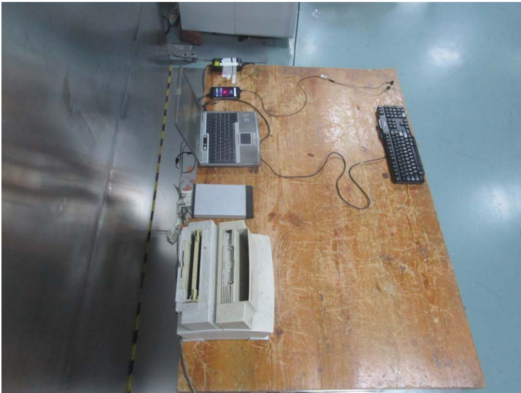
Conducted Emissions Side View
