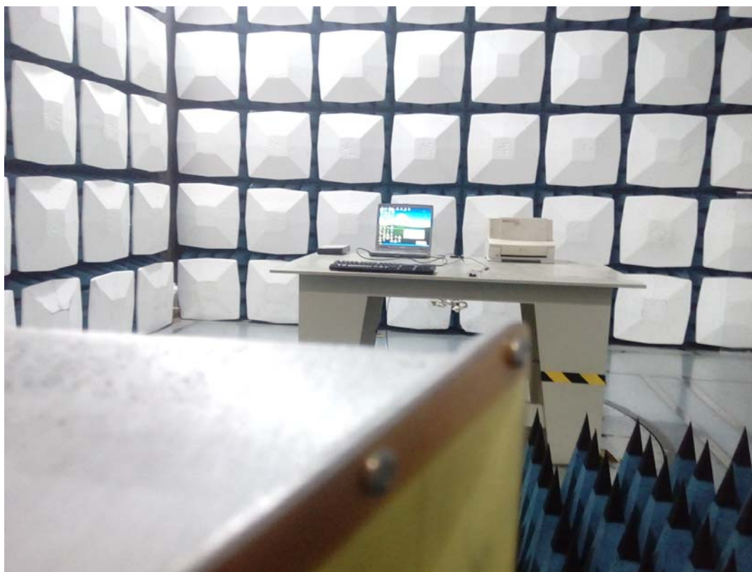
Radiated Emission Above 1GHz Rear View
