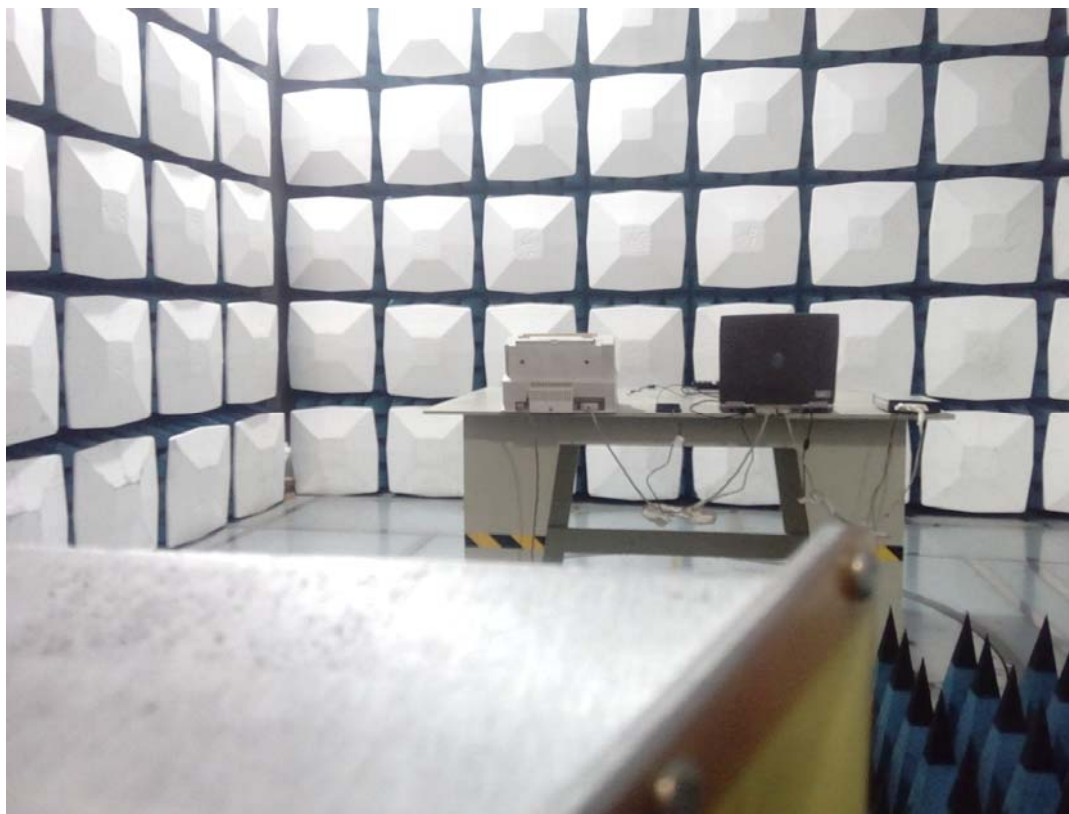
Radiated Emission Above 1GHz Rear View
