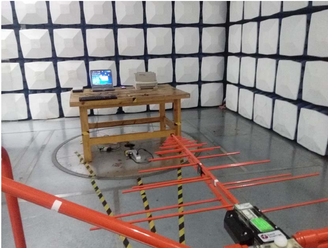
Radiated Emission Below 1GHz Rear View
