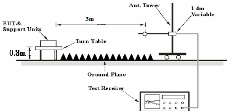
The radiated emission below 1GHz tests were performed in the 3 meters chamber test site A, above 1GHz tests were performed in the 3 meters chamber test site B, using the setup accordance with the ANSI C63.4-2014. The specification used was with the FCC Part 15 B Class B limits.
