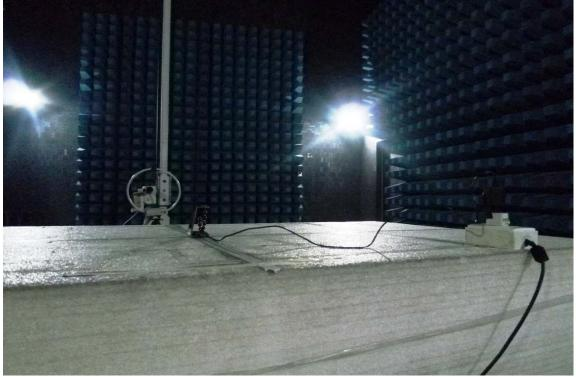
Radiated Emission Setup Photos (30MHz~1GHz)
