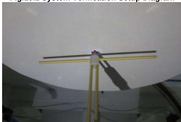
Fig.10.2 Photo of Dipole setup
