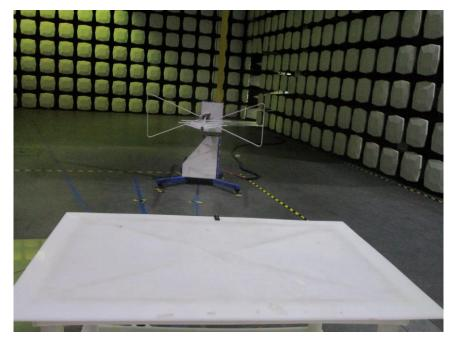
1.2 Radiated Emissions Test Setup
