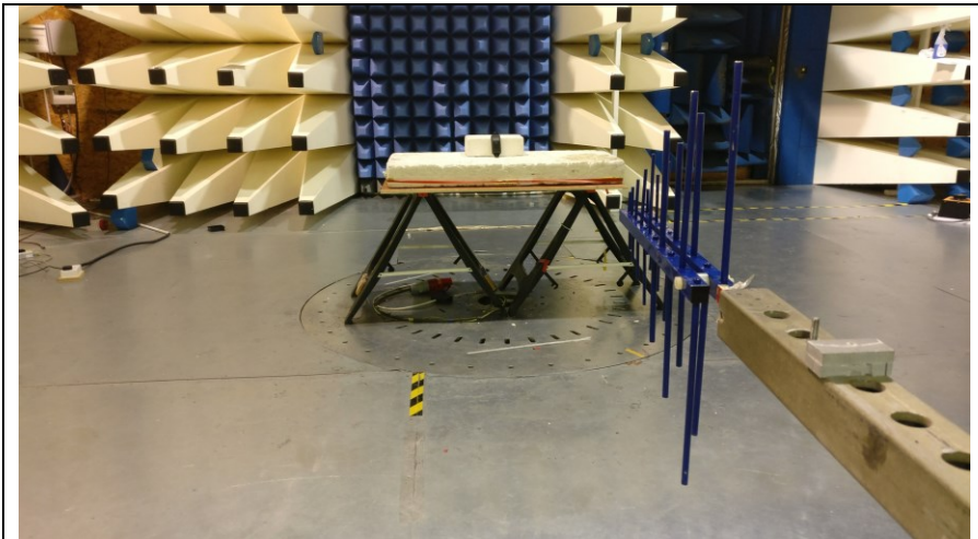
Fig 2b Test setup 300MHz -1GHz Rad Emissions
