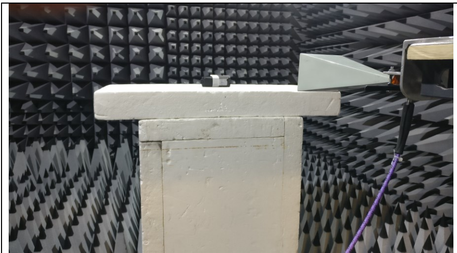
Fig 4 Test setup 18GHz -26GHz Rad Emissions
