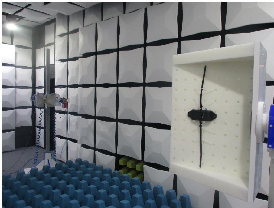
Test Setup: Radiated Measurements (1 GHz to 10 GHz)
