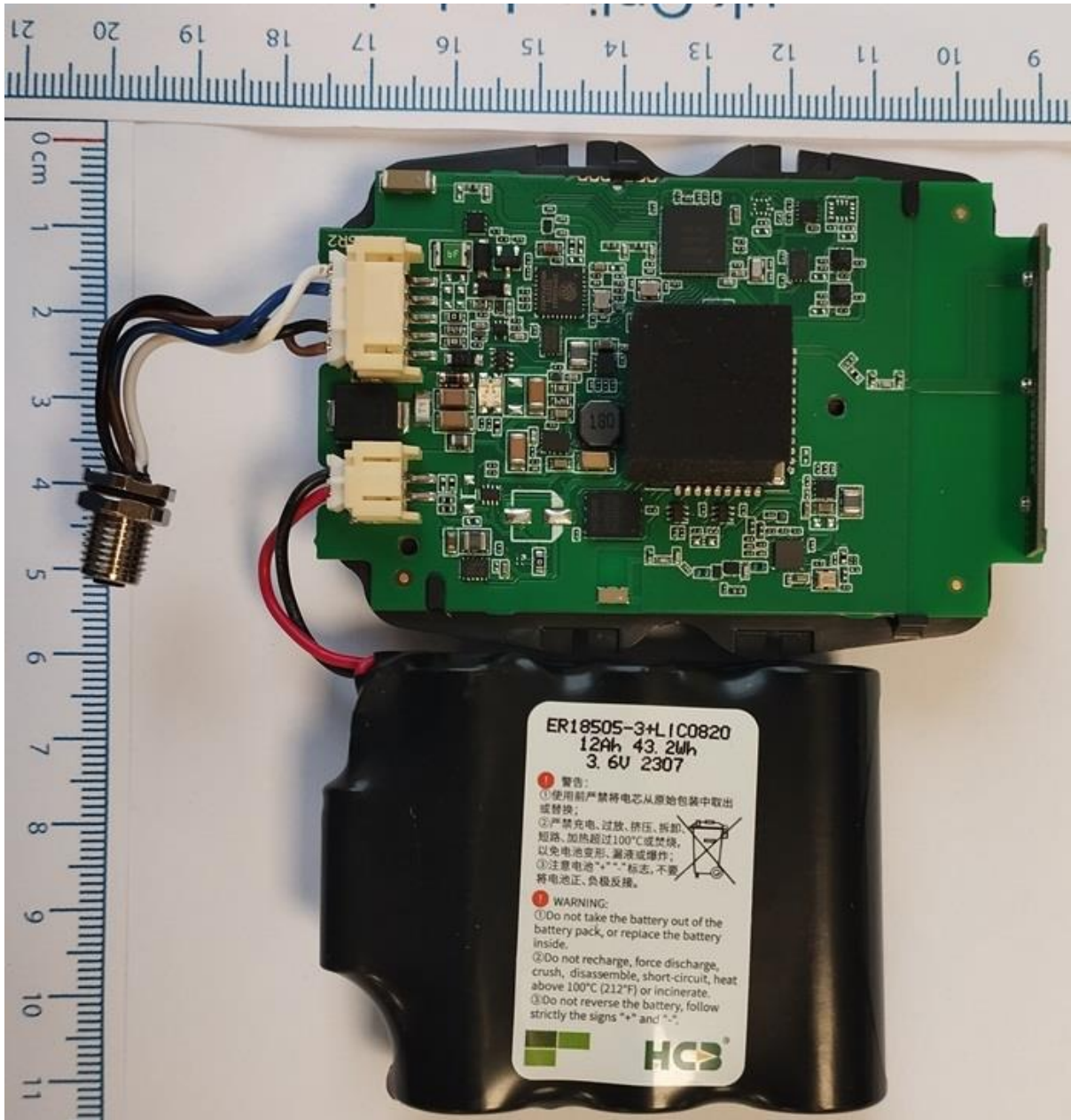
Figura 5: Side A - Hiti Battery- External DC power supply connector Hiti
