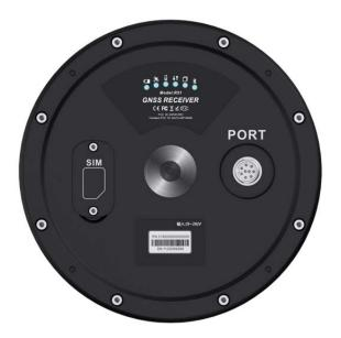
The bottom panel has a nine-pin aviation plug, 6 LED indicators, and a SIM card slot. In order to achieve IP67 waterproof level, the SIM card baffle is fixed with 2 screws
