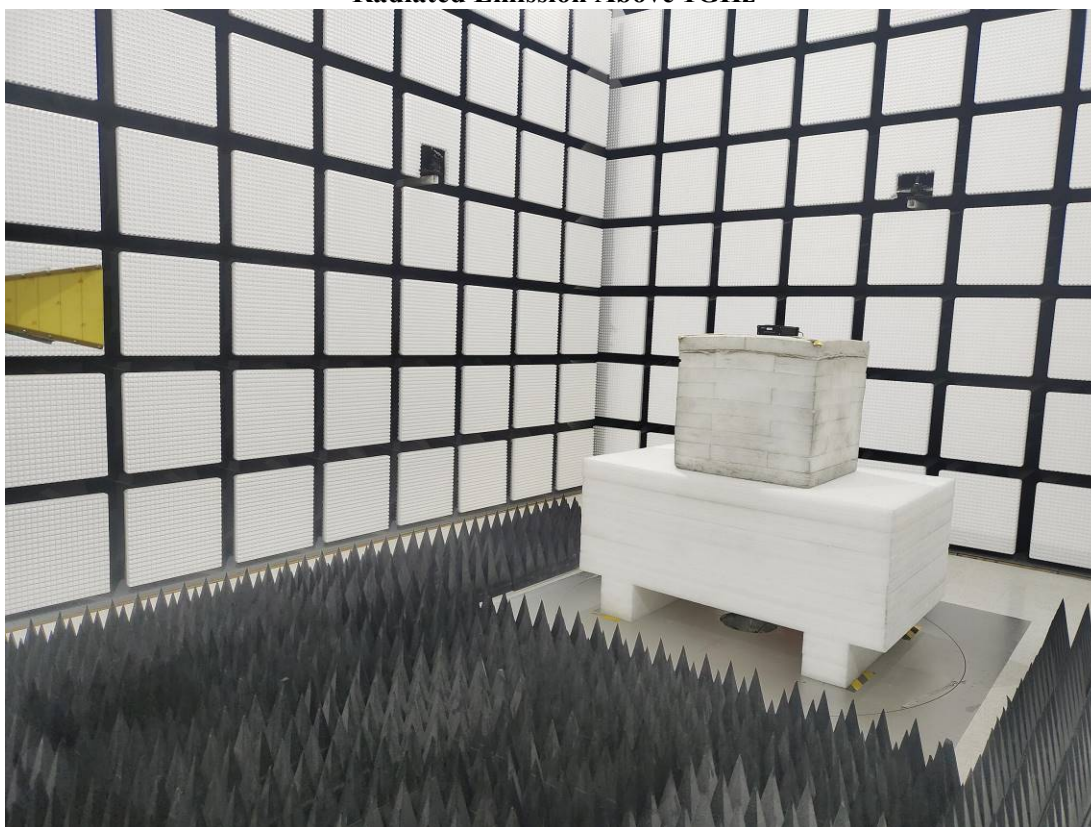
Radiated Emission Above 1GHz
