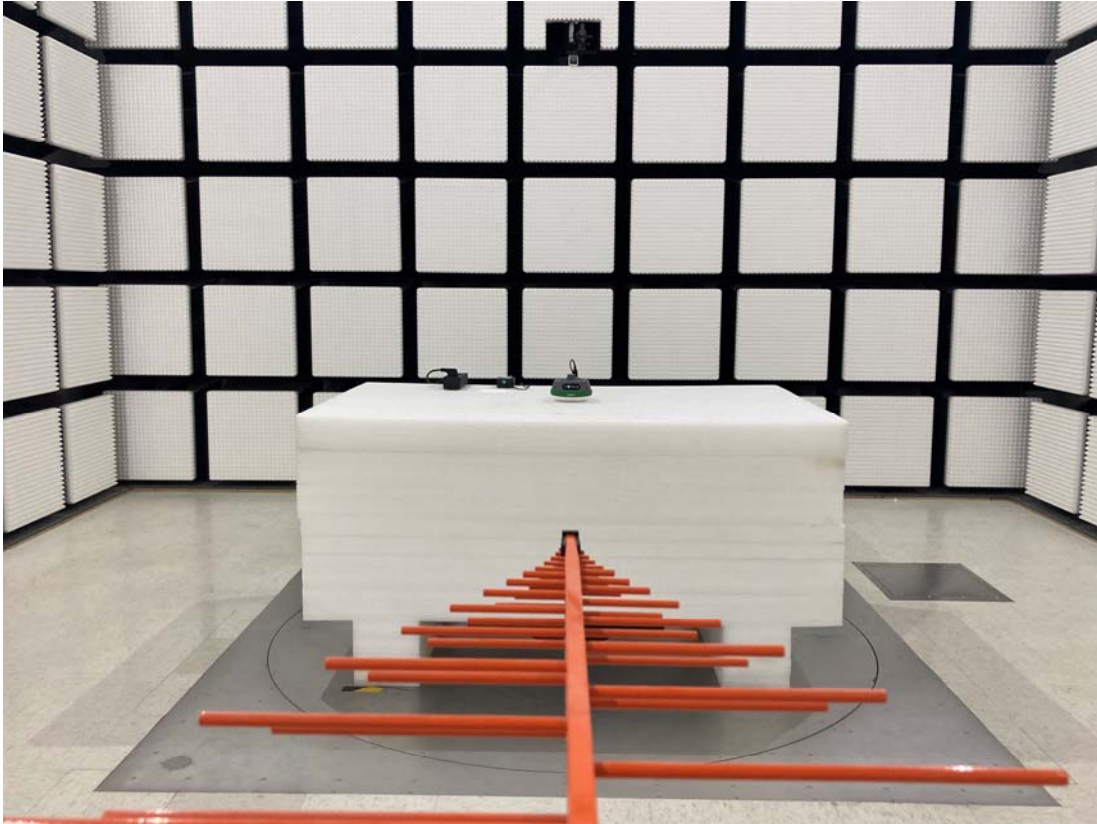
Radiated Emission Above 1GHz View
