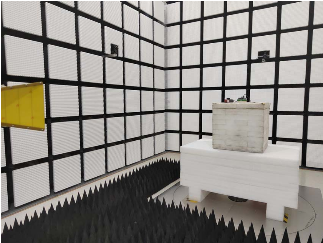
Radiated Emission Above 1GHz View
