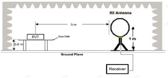
(2) Radiated Emission Test-Up Frequency 30MHz~1GHz
